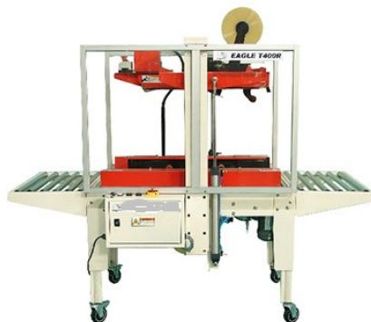
There are two basic types of case sealer. A semi-automatic sealer, which manually adjusts to different case sizes and a Random Case Sealer, which adjusts automatically. Both types can dramatically cut your labor costs.
